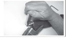
4. Remove the breech plug and the gun is ready for cleaning.
