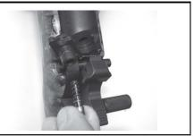
4. Remove the ramrod. Remove the screw on the underside of the receiver using a hex wrench.
