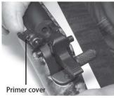
2. Using one hand to place pressure on the springloaded firing pin, use a small slotted screwdriver to pry the retaining clip from the primer cover
